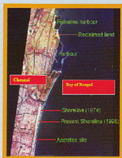
Fig.1. Erosion /Accretion along Chennai coast
